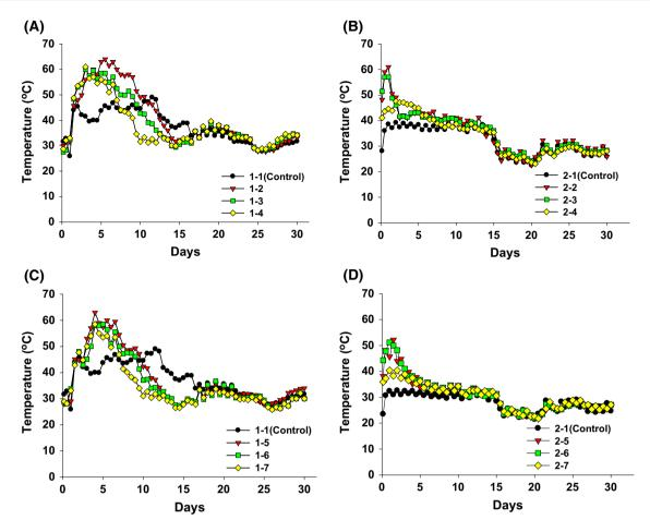
Fig. 2 Temperature profiles during successive VW composting cycles. (A) 1st cycle with SD, (B) 2nd cycle with SD, (C) 1st cycle with CP, (D) 2nd cycle with CP
