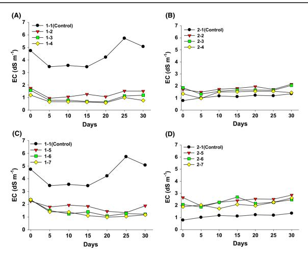
Fig. 5 EC variations during successive VW composting cycles. (A) 1st cycle with SD, (B) 2nd cycle with SD, (C) 1st cycle with CP, (D) 2nd cycle with CP
