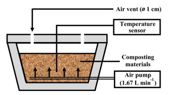
Fig. 1 Schematic diagram of a composting reactor
