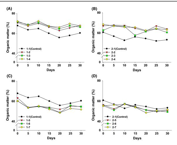
Fig. 6 OM content variations during successive VW composting cycles of (A) SD and (B) CP treatments
