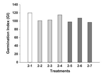
Fig. 8 Germination index (GI) of the final composts (GI < 80 indicates matured compost)
