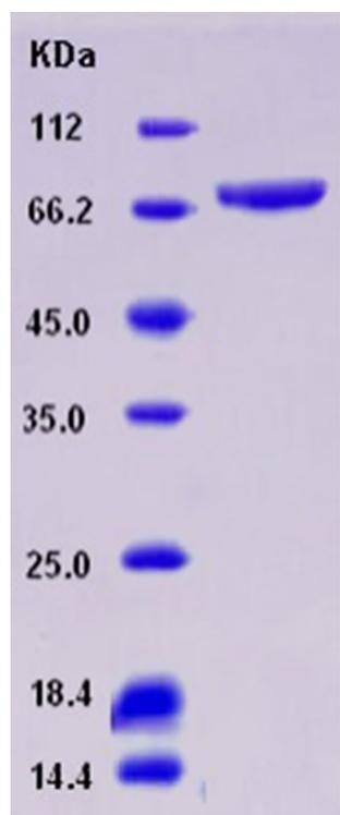
**Fig. 5** SDS-PAGE pattern showing the purification of the bovine liver TGase. Lane 1: Molecular Weight Markers, lane 2: purified TGase (74 kDa) from the gel filtration chromatography. The concentration of the separating gel was 10%. Migration was from top to bottom
