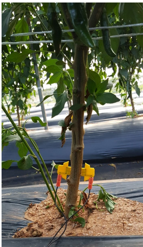
Fig. 1 Plant induced electrical signal (PIES) sensor inserted into the stem of pepper
