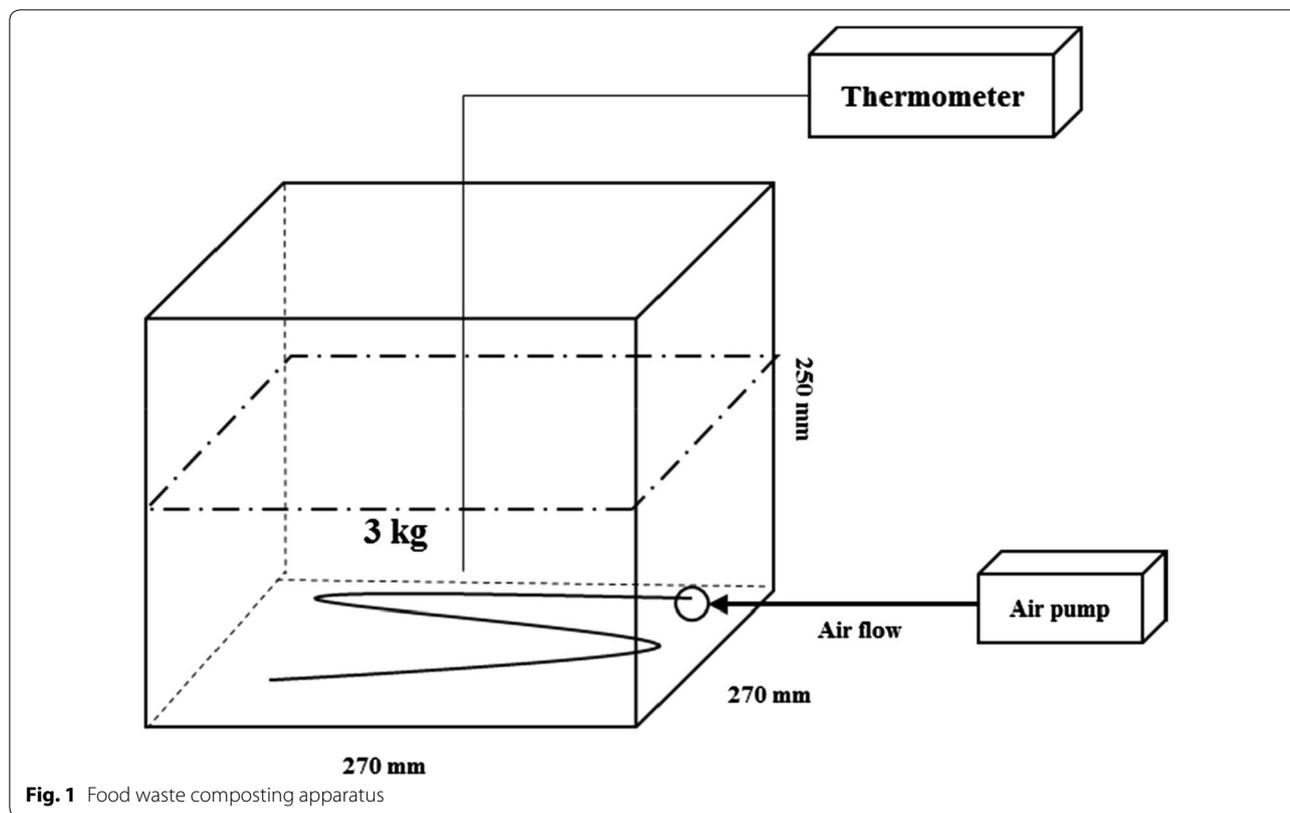
Fig. 1 Food waste composting apparatus
