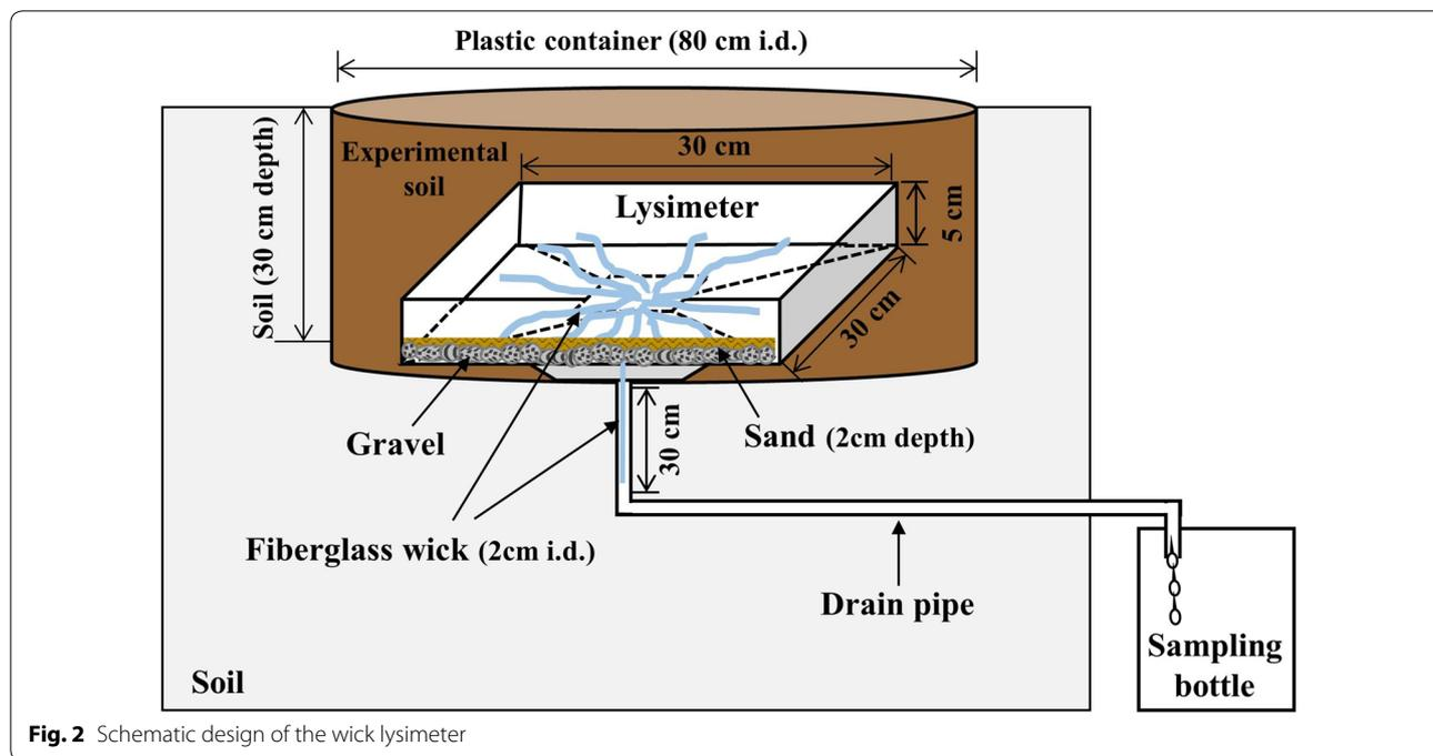
**Fig. 2** Schematic design of the wick lysimeter
